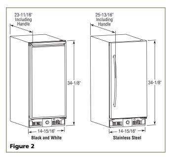
Please note that the unit has adjustable feet that can add one additional inch to height during leveling or to match adjacent cabinets (see **Figure 35** on **Page 14**).
